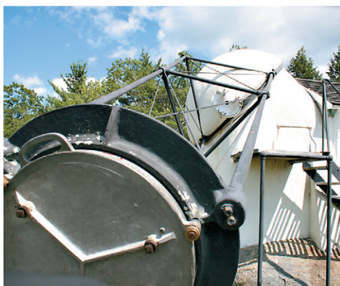
The primary cell (foreground), boom, and turret of the Porter Turret Telescope. Photo: Paul Varella
